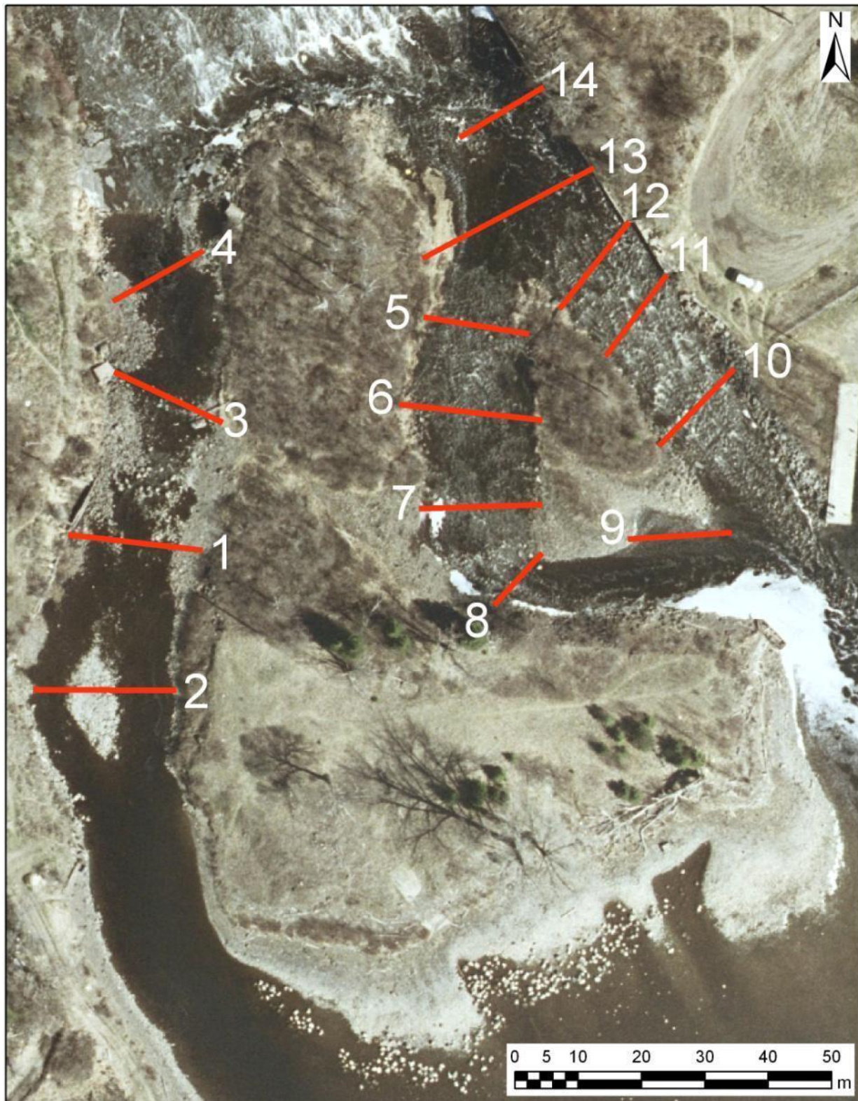
Figure 5. Location of substrate transects at the mouth of the Current River, September 2011. Note: City of Thunder Bay imagery date unknown (actual water levels were lower during sampling).
